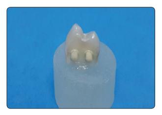
Fig. (2) Showing the tooth in acrylic block with the bonded sealers cylinders
