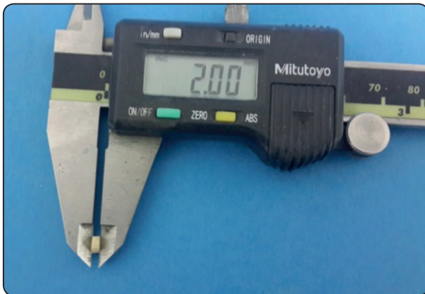
Fig (1) Showing 2 mm thickness recorded using digital caliper
