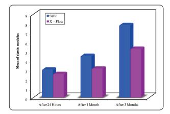
Fig. (1) Bar chart showing the comparison between the 2 groups according to elastic modulus.
