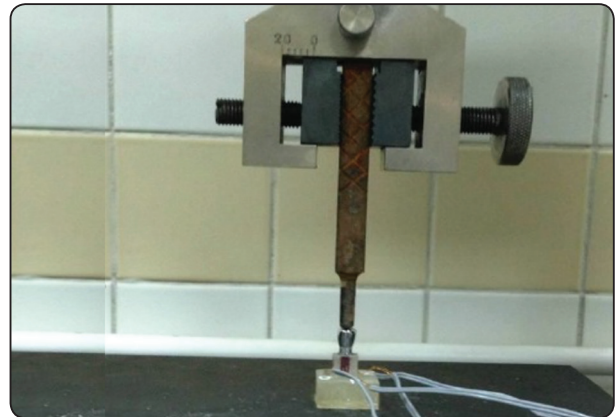
Fig. (3) Loading of the sample in the universal testing machine
