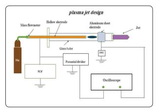
Fig. (1) A schematic diagram of the plasma device
