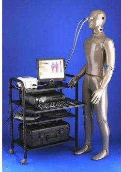
Figure.1 "Newton" thermal manikin
