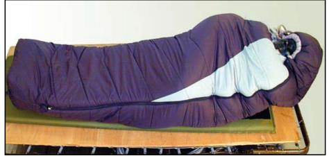
Figure 4: The articulated manikin, "Charlie 3", measures the thermal insulation of sleeping bags
