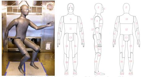
Figure 3. NEMO 23-zone submersible thermal manikin.
