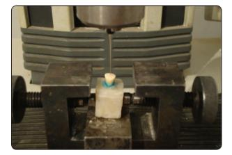
Fig. (1) Lloyd instrument testing machine (UK) when applying vertical force through finger plugger to an obturated root canal in composite mold up to fracture.
