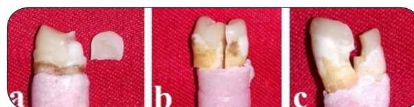
Fig. (9) The most common failure patterns; a) shoulder design showed 70-90% restorable fracture, b&c) butt joint and anatomical design showed 60-70% and 70-100% catastrophic fracture, respectively.
