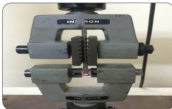
Fig. (1) Specimen under INSTRON universal testing machine.
