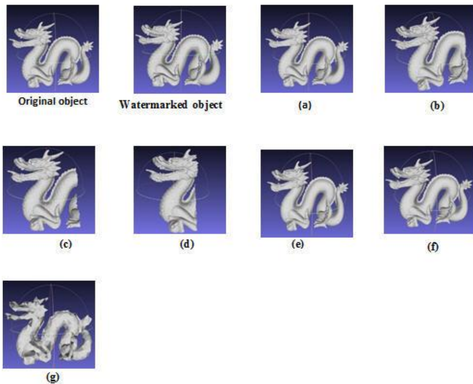
Figure 4: Original and watermarked dragon object before and after applying (a) Laplacian smoothing, (b) 10% cropping, (c) 30% cropping, (d) 50% cropping, (e) subdivision using midpoint scheme, (f) loop's subdivision and (g) simplification attacks.
