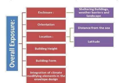
Fig.(6) The Design Parameters that affect the durability of the exterior finishing materials
