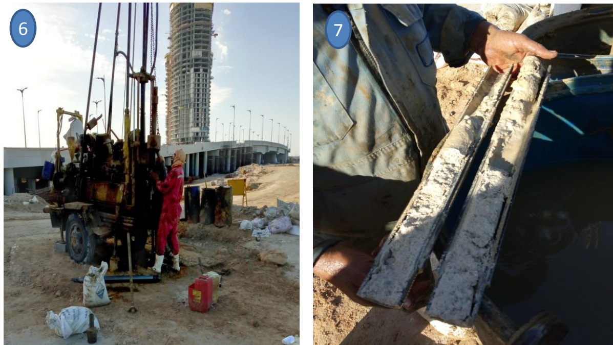
Figure 6 The Rotary drilling rig used for extraction of SPT samples shown in Figure 7 .
