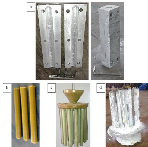
Figure 2 Photos of investment casting process: (a) a metallic wax injection die, (b) the produced wax samples, (c) wax tree and (d) the metallic tree after melt pouring and solidification.
