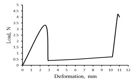
Fig. 2: Load vs. deformation for a persimmon fruit (destructive mode).
