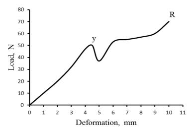
Fig. 4: Load-deformation curve for persimmon fruit samples in the parallel plate compression test.
