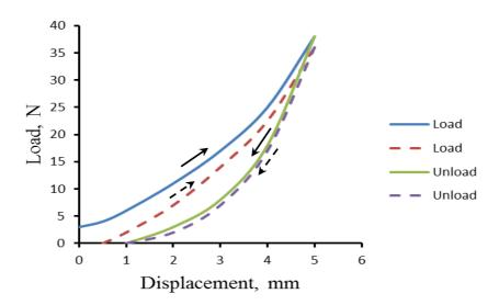
Fig. 5: Two successive load-displacement curves for anna-apple by using a 2-plates compressive test. The cycles include two loading and unloading stages.
