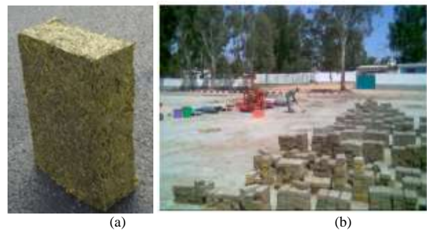
fig. 4. (a) Final straw-cement block (b) solid rice-straw based brick.
