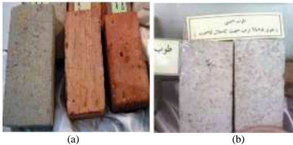
Fig. 6. HBRC New Bricks (a) Cement dust brick (b) recycled clay brick.
