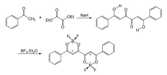
Fig. 3. Synthesis of tetraketone-based BF2 complex dye.
