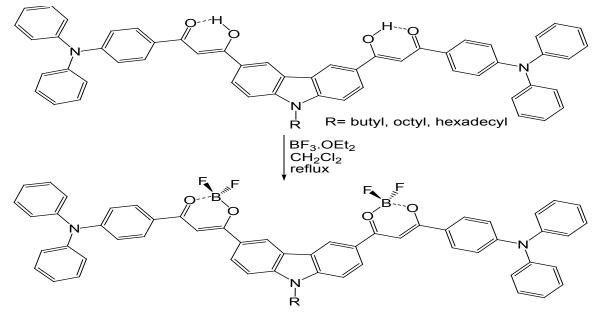
Fig. 6. Synthesis of bis(dioxaborine) carbazole complex dyes.
