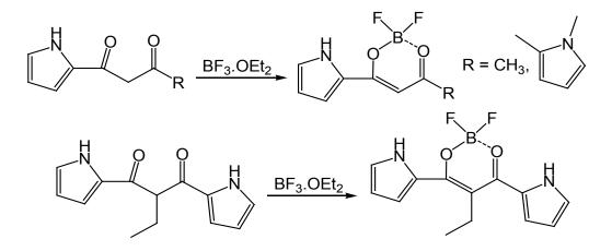
Fig. 9. Synthesis of BF2 complex derivatives from pyrrolyldiketones.
