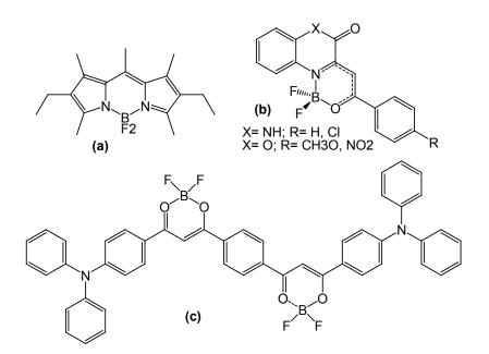
Fig. 1. Main classes of organic boron difluoride dyes depending on their ligand structure, including N-N doubledentate (a), N-O double-dentate (b) and O-O double dentate (c) ligands.
