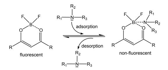
Fig. 4. Anticipated mechanism for the emission quenching upon exposure to volatile amines and its reversible process.
