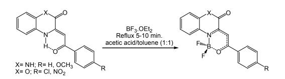
Fig. 15. Synthesis of boron difluoride complex derivatives containing arylethylidene-quinoxalin-2-ones or (arylethylidene)-benzo[1,4]oxazin-2-ones.
