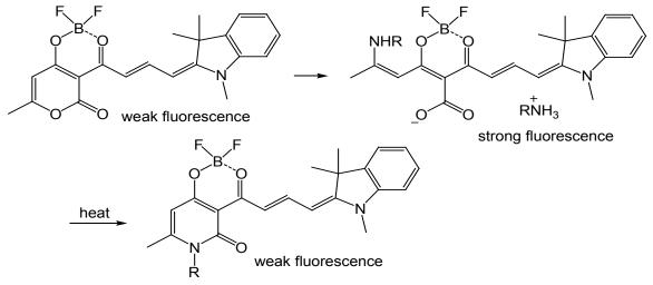
Fig. 5. Boron difluoride polymethine chromophore with low fluorescence with the ability to afford highly emissive open-chain chromophore, which upon heating cyclize to give pyridone with poor fluorescence.
