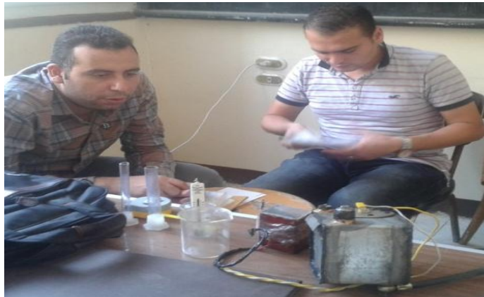
Fig. 5: Photo of calibration of fuel consumption assembly.
