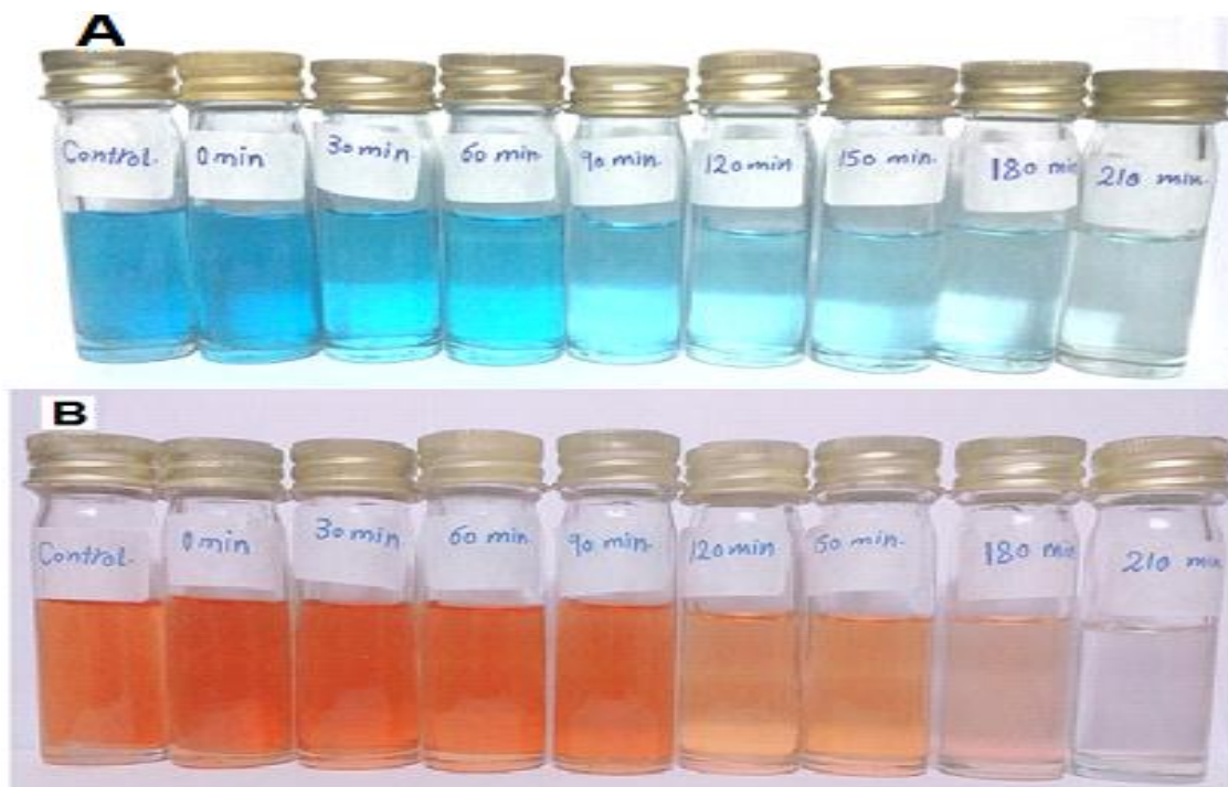
Fig.1: Photocatalytic activity of Alkalibacillus sp.w7 ZnO nanoparticles on (A) Methylene blue (MB) and (B) Methyl red (MR) as visually observed.
