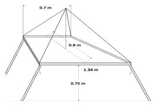
Figure (1) Schematic diagram of the solar still.
