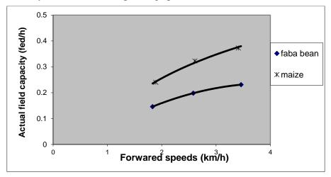
Fig. (12): Effect of different forward speeds on actual field capacity.
