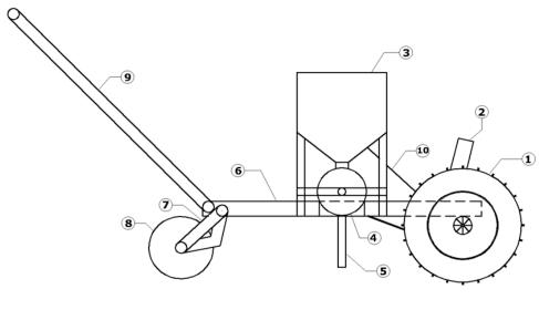
1.Drive wheels2. Furrow opener3.Seed box4.Housing of seed metering device5. Seed Tube6. Main frame7.Strips for install the path8. Rear wheel9. Push handle10. Transmission belt9. Push handle
