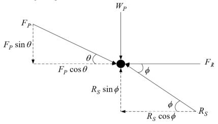
**Fig. 10:** Free body diagram showing all the forces acting on the single row planter
