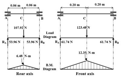
Fig. (8): The bending moment diagrams of the front and rear axis
