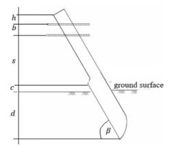
Figure 9. The main dimensions of the furrow opener
