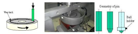
(a) Arrangement on sample (b) Geometry of a pin Fig. (3). Schematic of a pin-on-disc wear test and the arrangement of sample.
