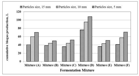
Fig.(5). Cumulative biogas production of different fermentation mixtures under different particles sizes.
