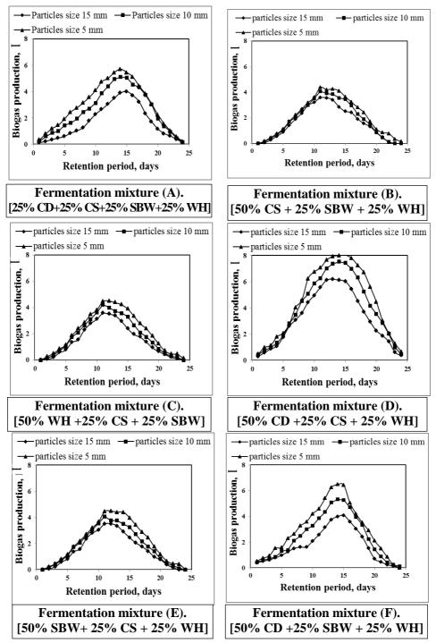
**Fig.(3).** Biogas production of different fermentation mixtures under different particles sizes.
