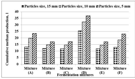
Fig. (8). Cumulative methane production of different fermentation mixtures under different particles sizes.
