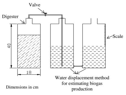
Fig. (1): The external view of the manufactured digester.
