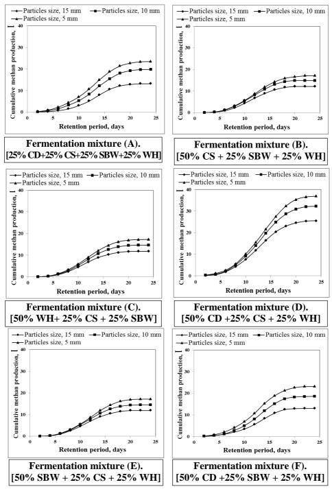
Fig. (7).Cumulative methane production of different fermentation mixtures under different particles sizes.
