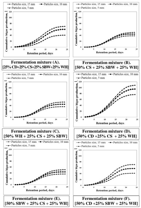
**Fig.(4).** Cumulative biogas production of different fermentation mixtures under different particles sizes.
