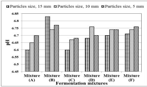
**Fig.(10).pH of different fermentation mixtures under different particles sizes.**
