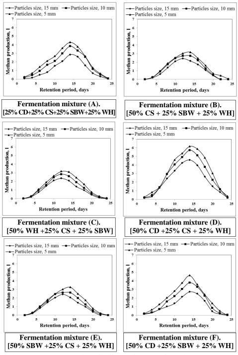
Fig.(6). Methane production of different fermentation mixtures under different particles sizes.
