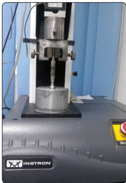
Fig. (2) Fracture resistance of cemented samples evaluated using Instron testing machine.
