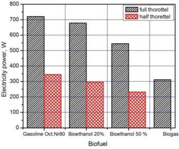
Figure 3: Present the electrical power generated from different biofuel during the operating of electrical generator.
