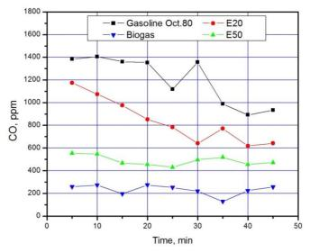
Figure 5: Concentration of CO produced from different biofuels during the operating of electrical generator at full throttle fuel position.
