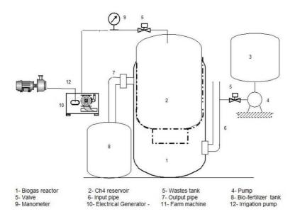
Figure 2: Biogas production unit and their component experimental set.
