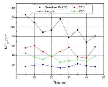
Figure 8: Concentration of  $NO_x$  produced from different biofuels during the operating of electrical generator at full throttle fuel position.
