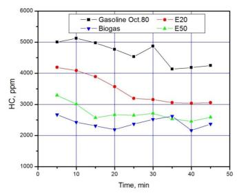
Figure 7: Concentration of HC (hydrocarbon gases) produced from different biofuels during the operating of electrical generator at full throttle fuel position.
