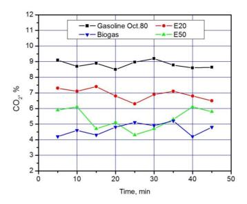
Figure 6: Concentration of CO<sub>2</sub> produced from different biofuels during the operating of electrical generator at full throttle fuel position.
