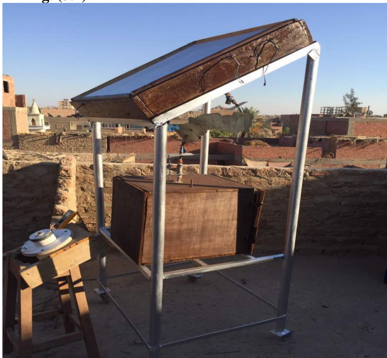
Fig.(3.1) Photograph of The solar powered adsorption refrigeration system setup.
