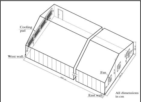
Fig. (1): Isometric view of rabbit house showing cooling pad with fans **1.3.The direct evaporative pad cooling system:**
