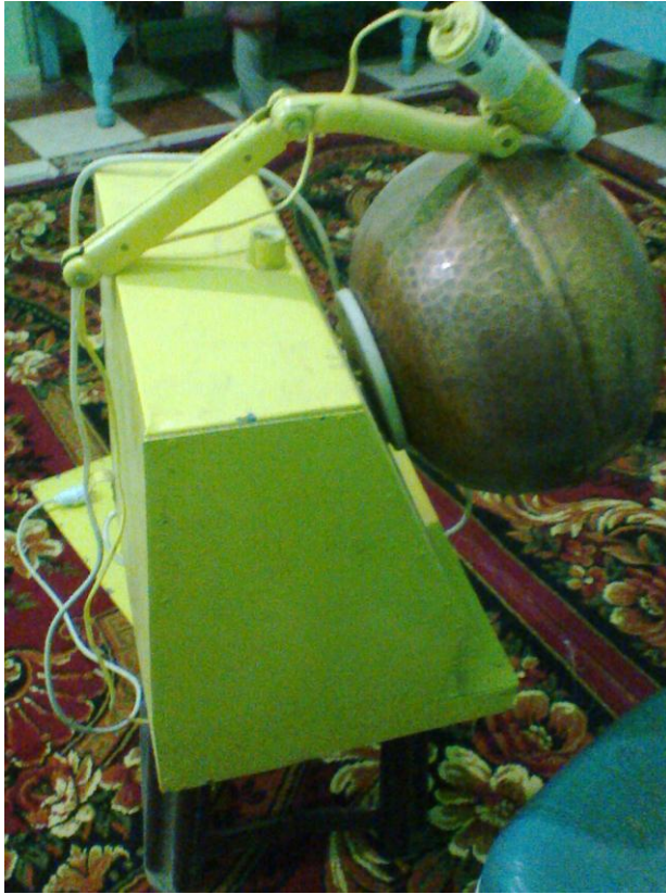
Fig. 2: Photograph of the seed-coating machine Abd-Al Fattah et al. (2015) and Abd-Al Fattah (2016).
