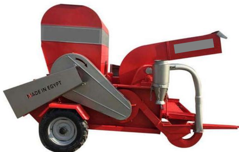
Fig. (1). The used thresher machine to chopping of the onion leafs.
