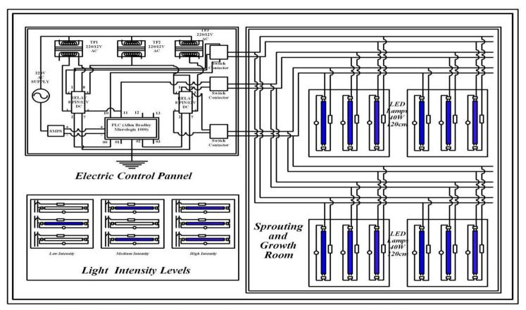
Fig. (5): Design of sprouting and growth room lighting system.
