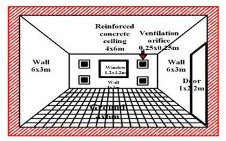
Fig. (1): Main dimensions of the chamber.
