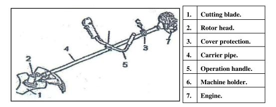
Fig (1): General view and main components of portable
