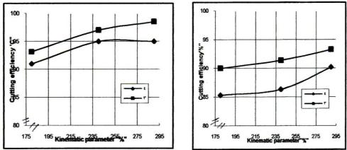
Fig (3): Effect of kinematic parameter"y" on the cutting efficiency "C" at different knife types and blade number.
