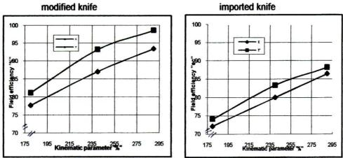
Fig (2): Effect of kinematic parameter"y" on the field efficiency "Ec" at different knife types and blade number.
