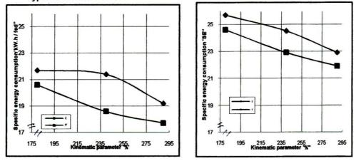
Fig. (4): Effect of kinematic "y" on the specific energy consumption "SE" at different knife types and blade number.
