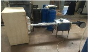
Fig. (1). Photo of the biogas dryer
