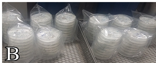
Fig. 1. Germination test procedure where (A) Seeds dispersal within petri dishes, (B) Allocation of petri dishes in the incubators.
