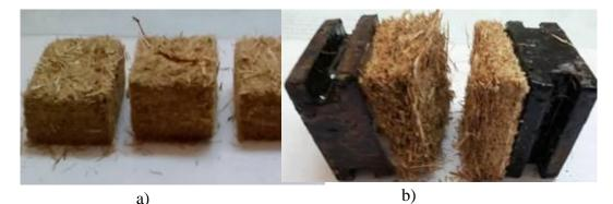
Fig. 2: samples for tension test, a) before the test. b) after the test.
