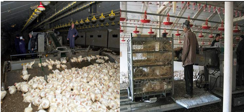
Fig. 3: CIEMME Super Apollo L catching machine while working.
