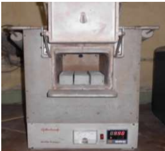
Fig. 1 Muffle furnace for post heating with tested prisms
