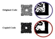
Figure 3: illustrate the copy-sensitive Seal-Vector code 2- Online FiberTag Technology:
