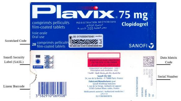
Figure 1: illustrate security features on SANOFI Plavix® package
