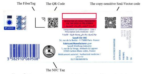
Figure 5: illustrate the suggested new digital anti-counterfeiting technologies
