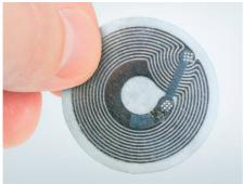
Figure 2: illustrate The NFC Chip The NFC Advantages:
