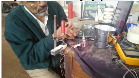
Figure (7). Primary tests on the amplifier for strain gauge.
