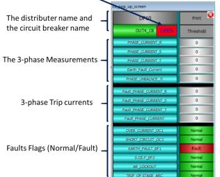
Fig.9. Protection relay screen (pop-up window)
