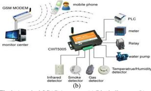
Fig.1. A typical SCADA system: (a) Block diagram, (b) Components.
