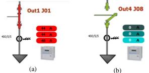
Fig. 8. symbolic figures of circuit breaker. (a) close state. (b) (Normal/Fault) open state.
