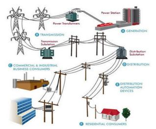
Fig.2. Electricity networks from generation to consumers.
