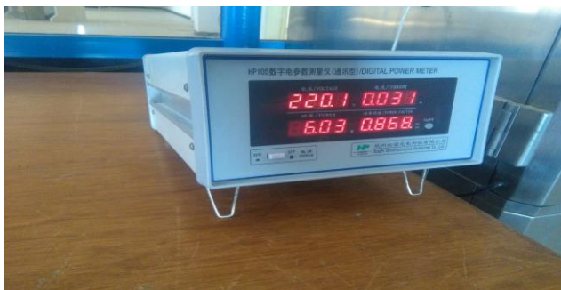
Fig.6. Digital power meter "HP105".
