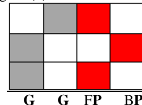
Figure (2) 3-Picks Weave Structure Technique used in the samples
