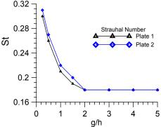
Fig. (13): Predicted Strouhal number for the two plates versus gap ratios,  $S_t = fh/U$
