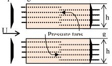
Fig. (1): Two plates model for surface pressure measurements
