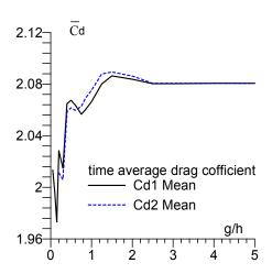
Fig. (8-a): Predicted time average drags coefficients acting on the two plates for different gap ratios g/h.
