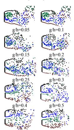
Fig. (10-b): DVM prediction of nearwake behavior for different gap ratio at normalized time t=300 nearly
