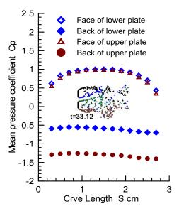
Fig. (9-a): Case of strong upward gap flow deflection – the base pressure coefficient is lower behind the plate in the deflection side.
