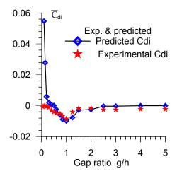
Fig. (8-b): predicted and experimental interference mean drag coefficients acting on the two plates for different gap ratios
