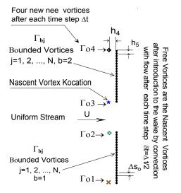
Fig. (2): Flow around two plate models prepared for numerical treatment as an inviscid model by modified DVM.
