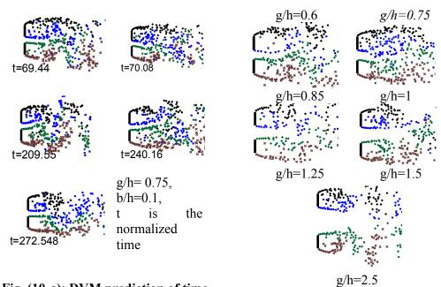
Fig. (10-a): DVM prediction of time variant near-wake behavior behind the two plates, g/h= 0.75
