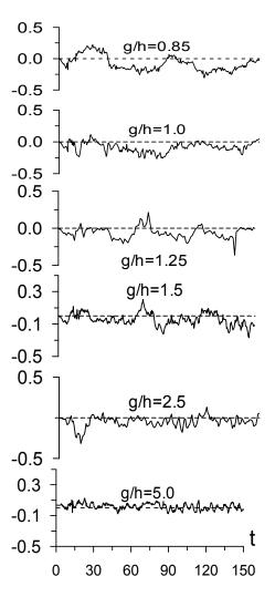
Fig. (12): Times variant interference drag coefficients  $C_{di}$  for different gap ratios g/h.  $C_{di} = C_{d1} - C_{d2}$
