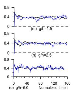
Fig. (11): time variant relative drag coefficient vs. gap ratio at normalized time equal 160 nearly  $C_{dr} = C_d - C_{d,single}$ ,  $C_{d,single} = 1.98$
