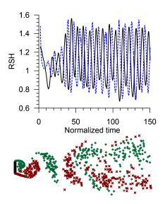
Fig. (4-b): Predicted characteristics of single flat plate b/h=0.1 by DVM with  $h_1=h_2=0.03$  - inside the intervals of independent solution.
