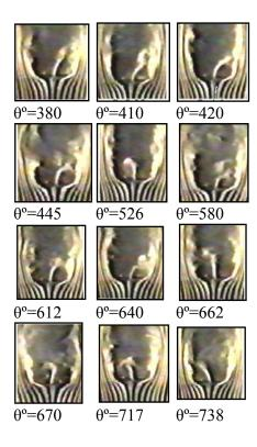
Fig. (5): Visualized time variant near wake behavior behind tow plates g/h=0.3,  $U_s = 2m/s$  and  $\theta^{\circ}$  is proportional with real flow time  $t_r$
