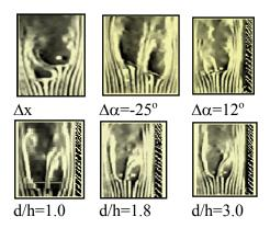
Fig. (6-b): Effects of asymmetric errors on the near-wake behavior g/h=0.8 for different d/h
