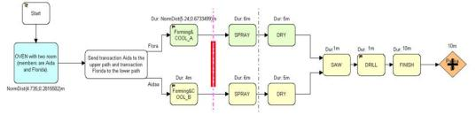
Fig. (2): The process map for ceramic factory.
