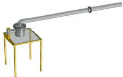
Fig. (5): the collection of impinged flat plate and its supported table as well as the real aluminum model
