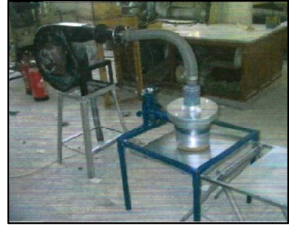
Fig. (7-b): Second available wind tunnel is used in the testing for lower mass flow rate range \dot{m} (0.2: 0.55 kg/sec)
