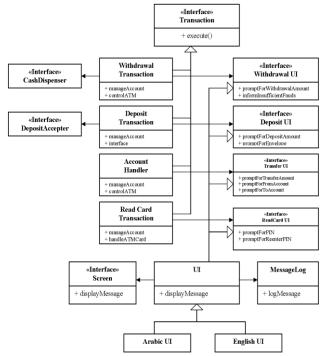
Fig. 18: A simple class diagram of the above ATM system [12]
