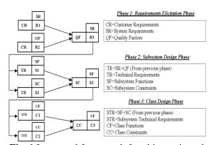
**Fig. 1** Integrated framework for object-oriented software development [8].
