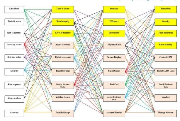
Fig. 17: Requirements traceability diagram for atm machine object oriented software design process.
