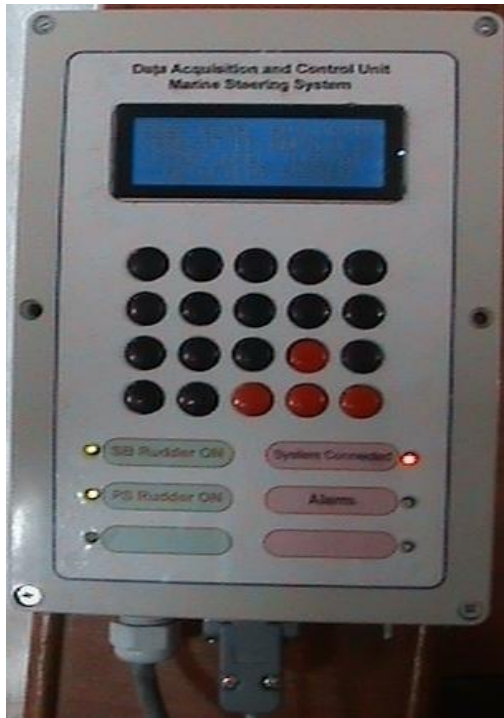
Fig. (15) The front panel of the data acquisition and control system DACS.
