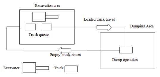
Fig. 1. Schematic outline of excavation operation
