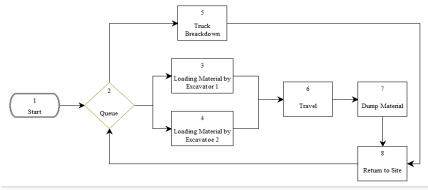
Fig. 5. Simulation model of excavation operation (case 2)
