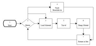
Fig. 2. Simulation model of excavation operation (case 1)
