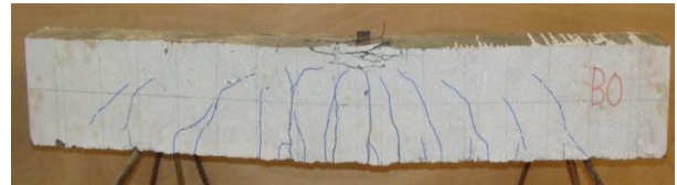
Fig. (6) Mode of failure of tested beam B0
