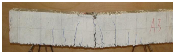
Fig. (5) Mode of failure of tested beam A3
