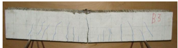
Fig. (7) Mode of failure of tested beam B3
