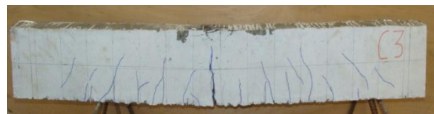
Fig. (9) Mode of failure of tested beam C3
