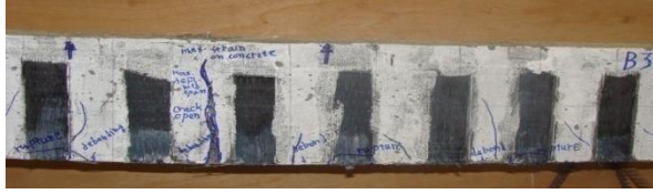
Photo (10) Mode of failure of tested beam B3-S12
