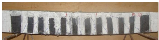
Fig. (9) Mode of failure of tested beam B0-S12
