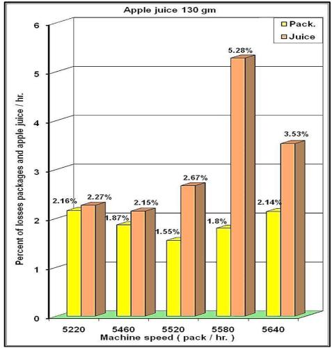
FIG.(8): Comparison between different rat of (VP. 240, 130 gm), damaged packages and losses apple juice in plant ( B ).
