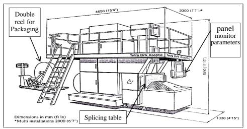
Fig. (1): Tetra brick aseptic packaging machine (Type: TBA/19-010V)
