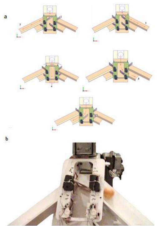
Fig. 3 a: Schematic view and b: photograph of arrangements of grading gates and grading paths
