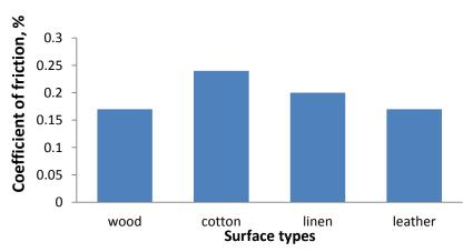
Fig. 4 Coefficient of friction for Valencia orange on wood, cotton, linen and leather
